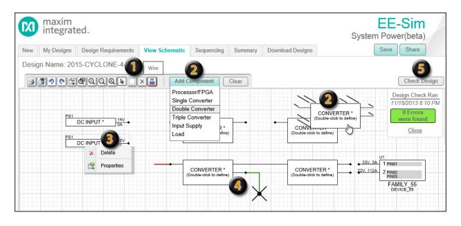
**Toolbar**: The top of the window shows a toolbar including familiar commands such as print, undo, redo, zoom, select, delete, and wire commands. Position your mouse over an icon to view its functional name in a tooltip.
