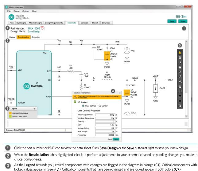
Double-click or right-click a component to edit its properties or change vendors. Critical components feature an orange banner at the top of the properties window. A component shows its locked or unlocked state with a checkbox on the properties window and a padlock icon that appears in the locked or unlocked state.
