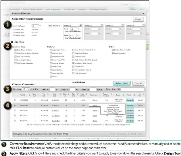
Apply Filters: Click Show Filters and check the filter criteria you want to apply to narrow down the search results. Check **Design Tool** Available to find solutions that feature the EE-Sim DC-DC Converter Design tool. Click **Hide Filters** to stop showing the filter criteria and simplify the appearance of the page.
